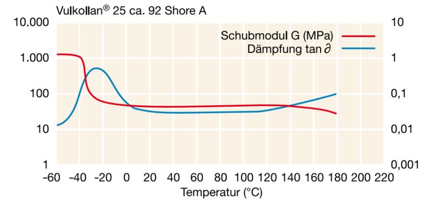
Solid Vulkollan® stiffens as the temperature falls (below -10°C). The glass transition temperature is approximately -40 °C, but embrittlement only sets in at much lower temperatures.
