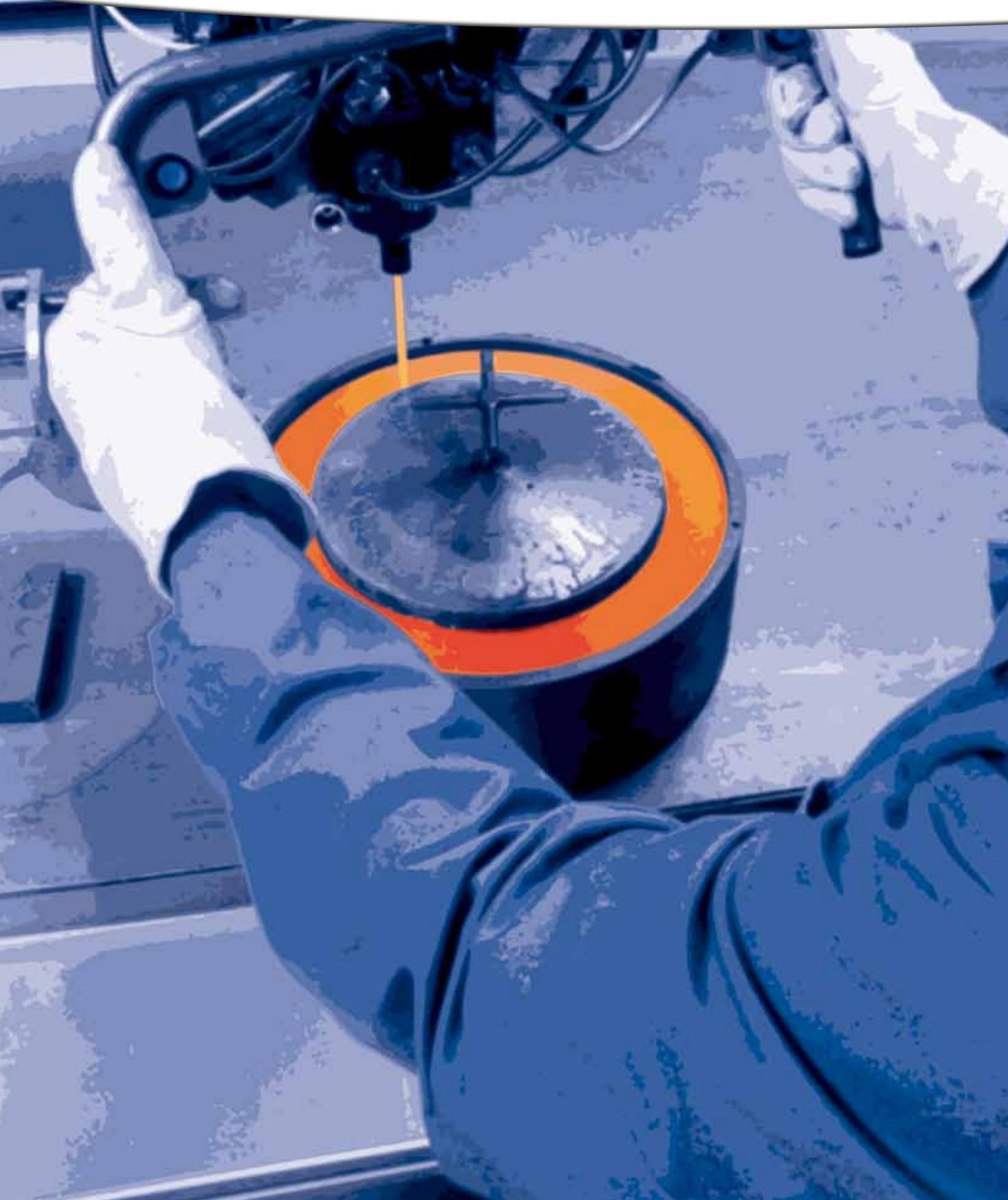
Vulkollan® is a high-grade polyurethane elastomer based on raw materials from Bayer MaterialScience: Desmodur® 15 and special polyester polyols. The rubber-elastic material boasts outstanding mechanical load-bearing properties and dynamic load resistance.
